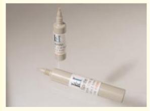
Direct connect Sprite HPLC columns require no tools for leak-free finger-tight operation.
